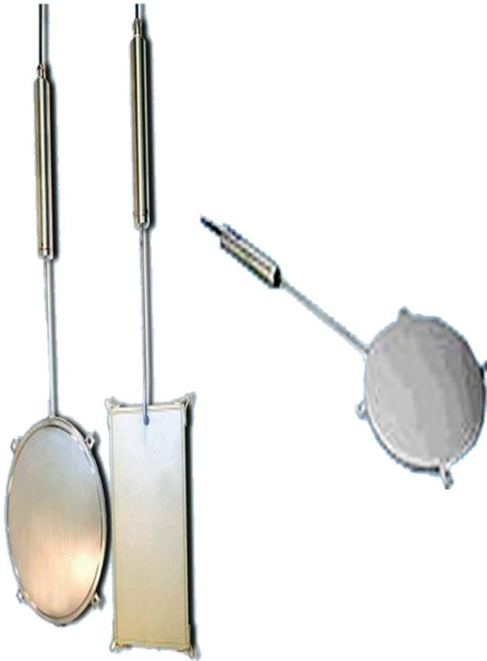
Model SIS-1100 Series Total Pressure Cells are used to measure total pressure in soils and embankments, at the interface of two different materials or measurement of stress in concrete. They are also used for measurement of contact pressures on retaining walls, buildings, bridge abutments, tunnel linings etc.
